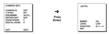
Caution: If you use an infrared light source while in AUTO mode, AUTO switching malfunction and camera AF malfunction may occur.
